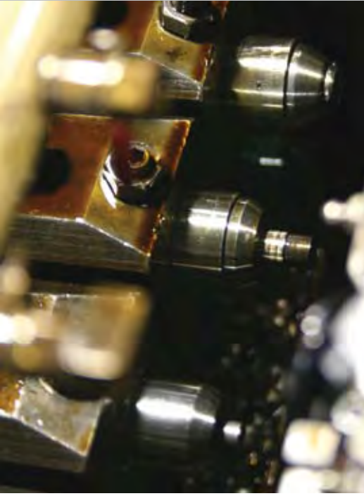
Closeup of punches in a multi-die header. (Reed & Prince Manufacturing Corporation. Photo by Jean Butler.)
