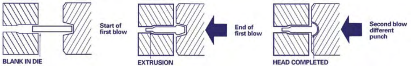
Above Photo: The typical one-die, two-punch method is common in producing headed parts, especially fasteners. The first blow combines partial head upset (coning) with shank extrusion. Then the second blow finishes the head shape. (Illustrations courtesy of Carpenter Technology Corporation.)
