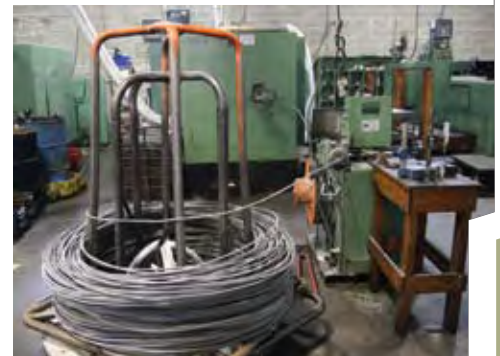
Wire from a coil is pulled through a carbide draw die that sizes it to a precise diameter. From there, the wire feeds into a 4-die header. This machine was producing parts that would later be finish machined at the customer’s shop. It was running at the rate of 70 parts per minute. Other machines in the plant make different parts at up to 200 or more parts per minute.
